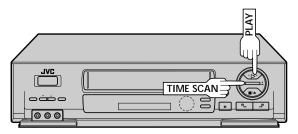
Your VCR is equipped with the TimeScan function. TimeScan allows noise free pictures to be displayed on your TV screen in the forward and reverse search modes. Audio will be played back at normal speed during any of the TimeScan modes (F) pg. 37). TimeScan allows you to view a program in search mode while listening to the audio.
